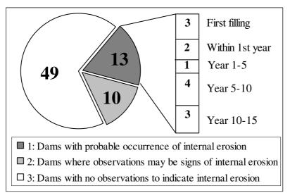
Figure 2. Number of dams and elapsed time until first internal erosion sign.
