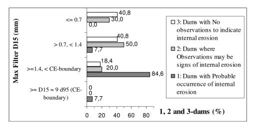
Figure 3. Filter D15-distribution in relation to performance history of internal erosion (dam categories 1-3).
