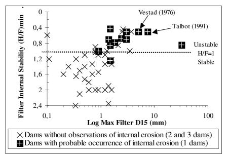
Figure 4. Filter D15 put against filter internal stability in relation to performance history of internal erosion (dam categories 1-3).
