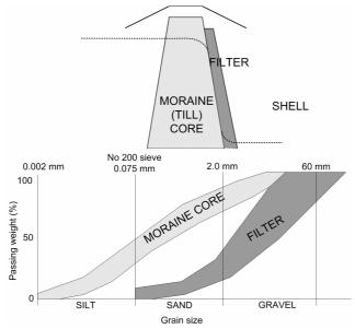
Figure 1. Typical cross-section of moraine core dams and typical sieve curves of widely graded material of glacial origin.
