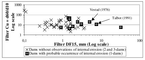
Figure 5. Filter D15 put against coefficient of uniformity (Cu) of the filter in relation to performance history of internal erosion (dam categories 1-3).
