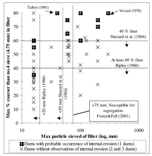
Figure 6. Percentage coarser than no. 4 sieve in filter put against maximum particle sieved in filter in relation to performance history of internal erosion.
